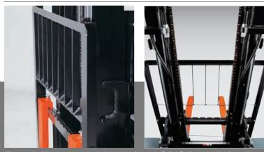
The angled lower stay ensures a good view of the fork tips, which makes it easier to insert forks into the pallet on the ground.
