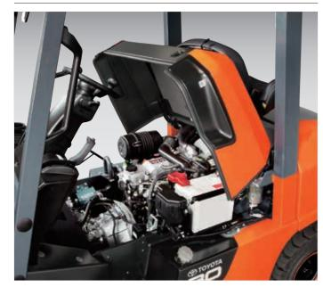
The wide-opening engine hood supports easy access to the engine compartment for inspection or servicing.
