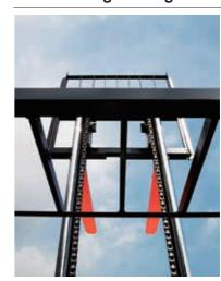
The headguard uses a lattice design that combines outstanding upward visibility and strength.
