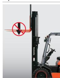
When the key is switched off the forks do not descend even if the load-handling levers are operated. This can help prevent accidents caused by unintended operation by someone other than the operator.
