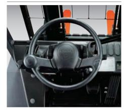
The small-diameter steering wheel teams up with the full hydraulic power steering system to provide excellent maneuverability. The steering column offers stepless adjustment to accommodate a wide range of operator preferences.
